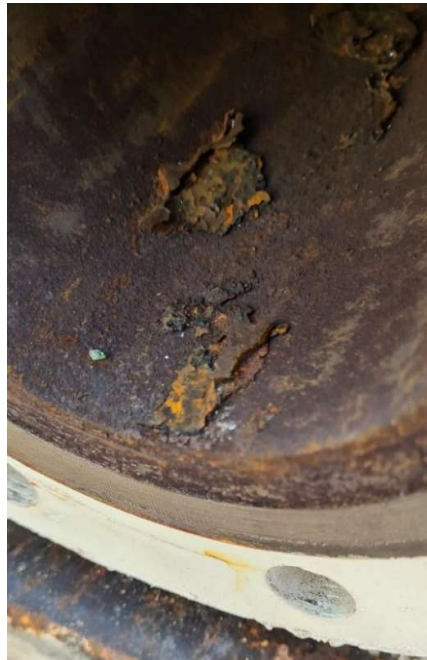
Figure 20. Meter As Found With Corrosion Induced Fouling
