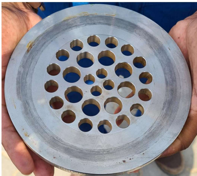
Figure12. Removed Flow Conditioner with Light Rust Dusting
