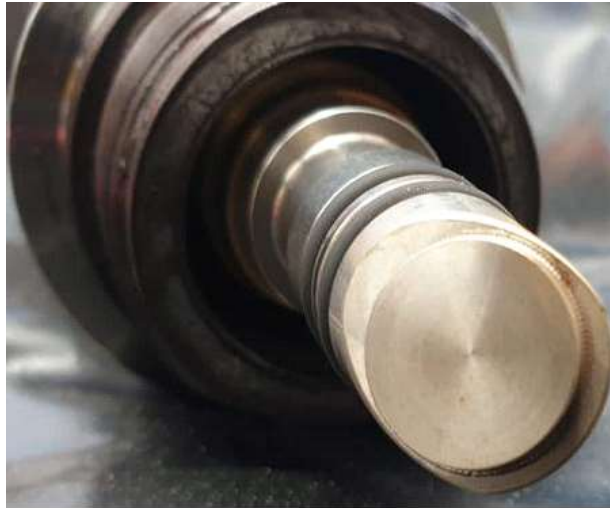
Figure 13. Removed Flow Conditioner with Light Rust Dusting
