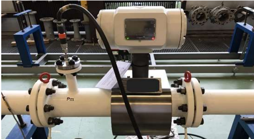
Figure 3. The 4" Honeywell Q Sonic-Max 8-path Ultrasonic Meter Installed at Calibration Facility.
