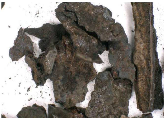
Figure 11. Rust Particulate Removed from Inside of Meter
