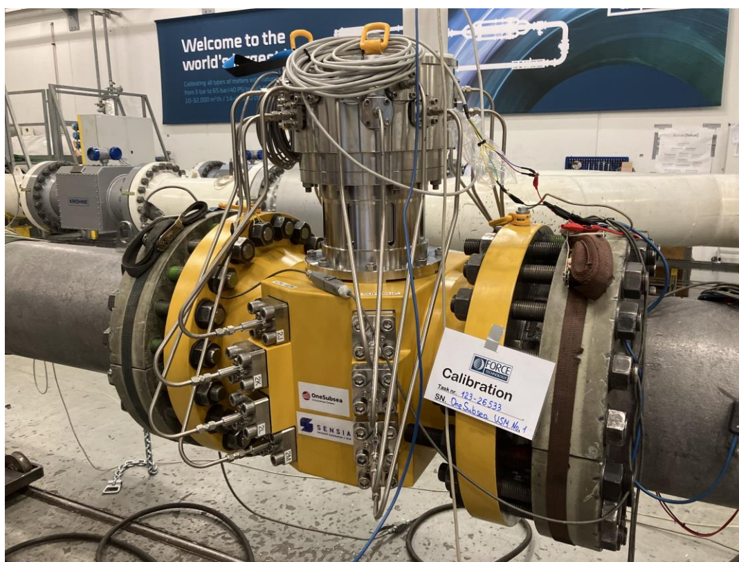
Figure 16 – The 8-path 16-inch subsea ultrasonic flowmeter installed in FORCE Technology's calibration test facility.
