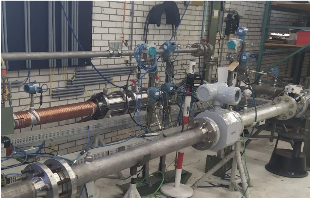
Figure 7: The 4" ALTOSONIC V12 ultrasonic custody transfer gas flowmeter installed at the DNV hydrogen test facility.
