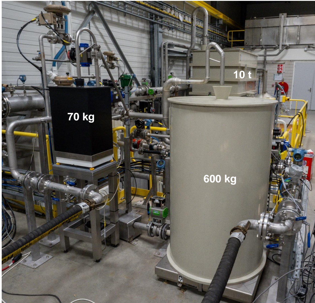
Picture 2 – The weighing instruments with holding tanks (70 kg, 600 kg and 10 t)
