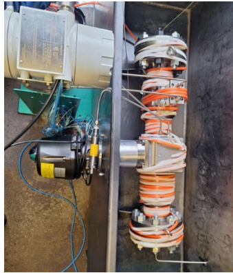
Fig 7 & 8. Test meter wrapped in heating cable and thermal insulation.
