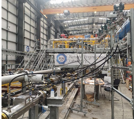
Fig 4. Optimum installation of impulse lines
