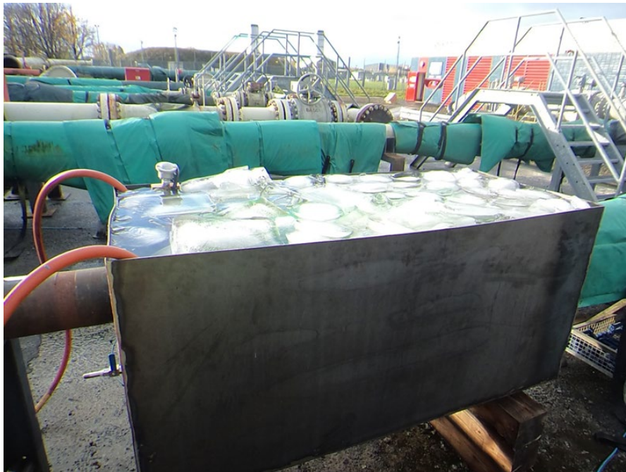
Figure 5 - Carbonstream meter installed in ice bath at DNV Bishop Auckland
