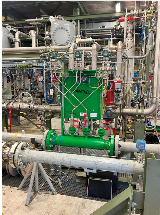
Figure 7 - "Topside" Carbonstream mounted in DNV Groningen loop for CO2MET JIP
