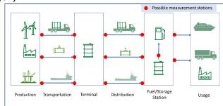
Metering technologies Measurement station concept
