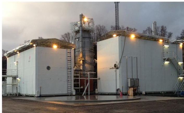
Figure 7 The compressor performance test loop. A simplified Process Flow Diagram indicating the position of the Subsea Ultrasonic Flowmeter to the left, and a photo to the right. The compressors are placed on the circular concrete slab in the front. This forms the bottom of a large water tank with a removable wall so that the compressors can be submerged during testing, see Figure 8 .
