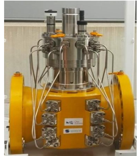
Figure 2 A 16-inch subsea ultrasonic flowmeter.
