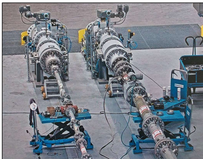
Fig. 1: Hydrogen calibration of an 8"/DN200 flowmeter.
