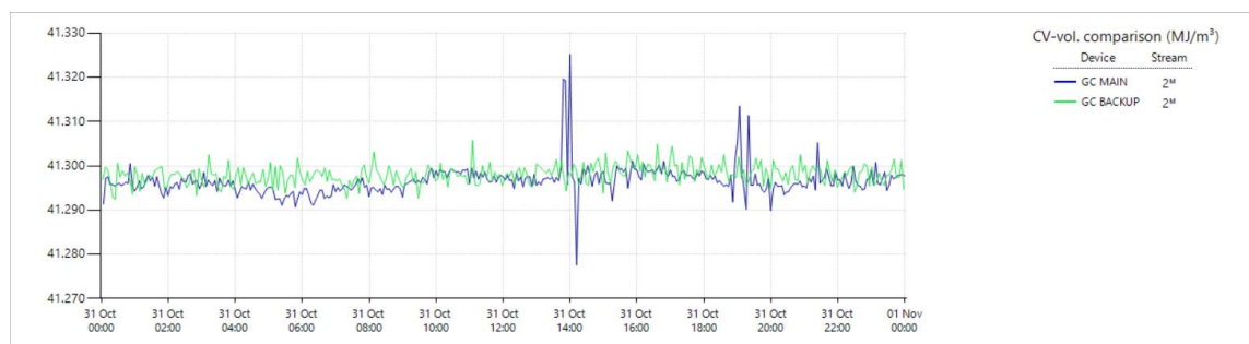
Figure 14. Duty / Standby GC CV comparison on BGP
