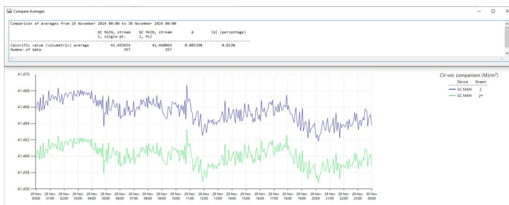
Figure 3. Bias due to GC non-linearity (MLC vs single point calibrated CV)
