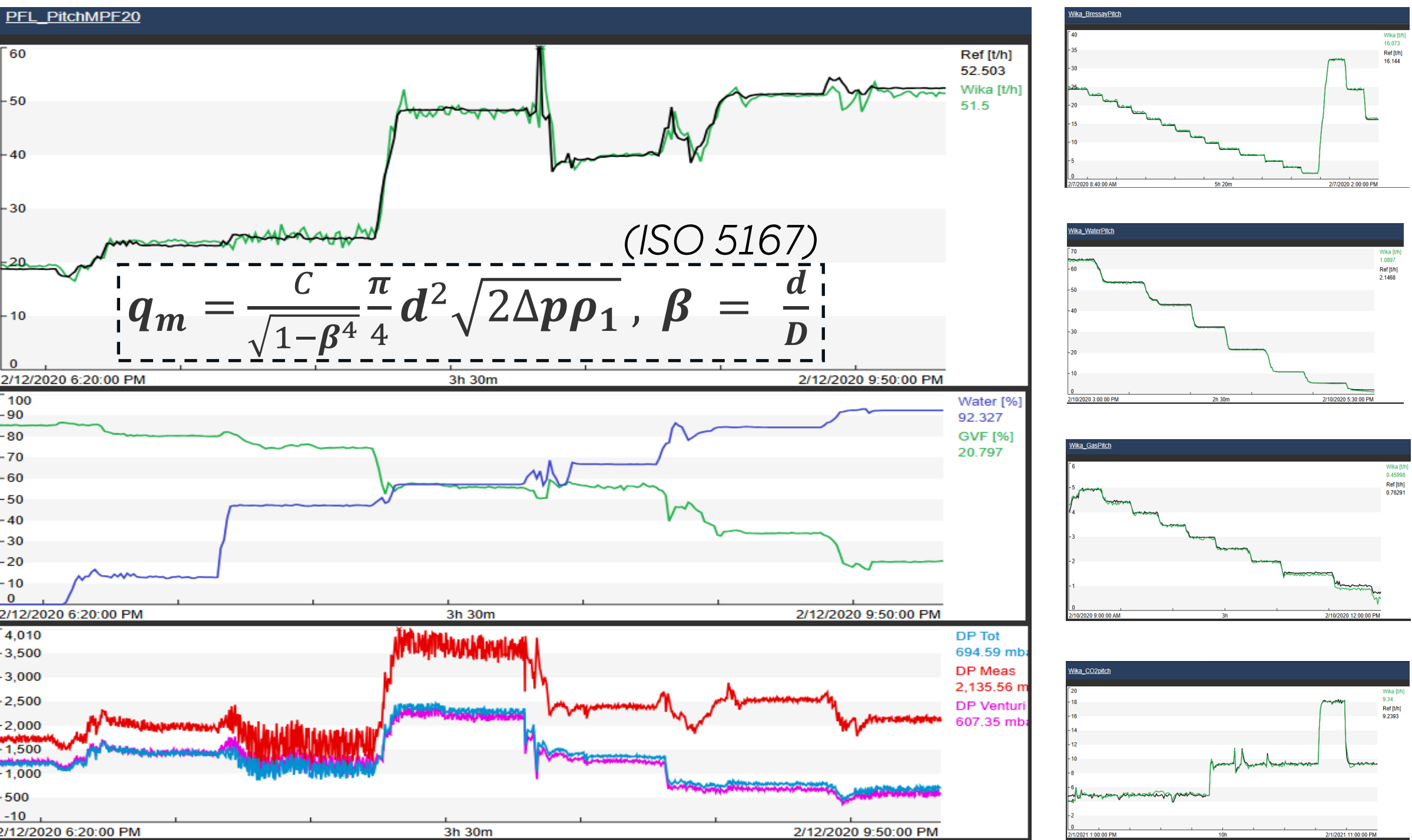
Multiphase flow loop test data with reference (black) and differential pressure flow meter (pink) rates in the upper plot. Water Liquid Ratio increased from 0 to 92 % (blue line, second plot) and GOR was around 100 Sm 3 /Sm 3 . The third plot shows mixed density (gamma densitometer, green dashed line) and the measured differential pressures from the flow meter used to calculate flow rate
